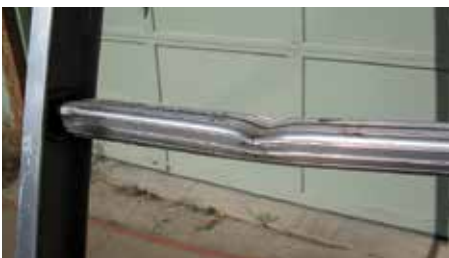
Ladders with defective parts, such as this broken rung, shall be removed from service.
